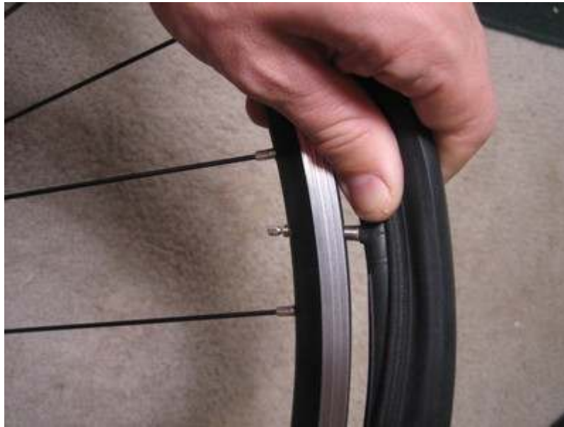
Remove the valve stem from the rim. (c) David Fiedler, licensed to About.com
