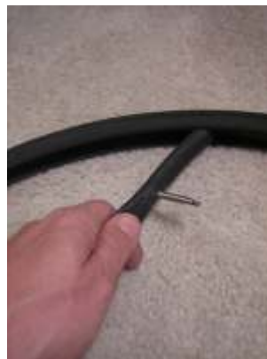
Remove the old tube from the tire. (c) David Fiedler, licensed to About.com
