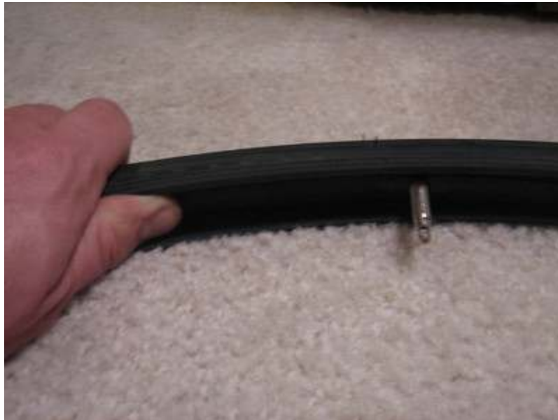
Place the new tube in the tire. (c) David Fiedler, licensed to About.com
