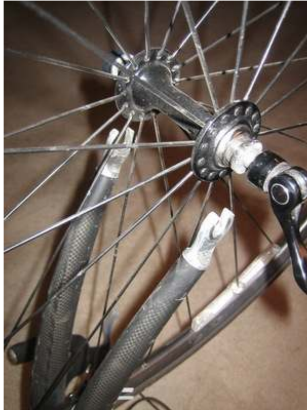
Replace the wheel on the bike. (c) David Fiedler, licensed to About.com
