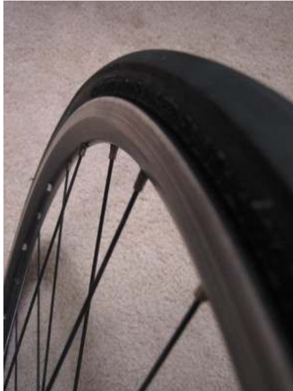
Here's the way the tire should look properly seated on the rim. (c) David Fiedler, licensed to About.com
