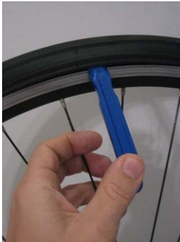
Replace the tire on the rim, using tire tools when necessary. (c) David Fiedler, licensed to About.com
